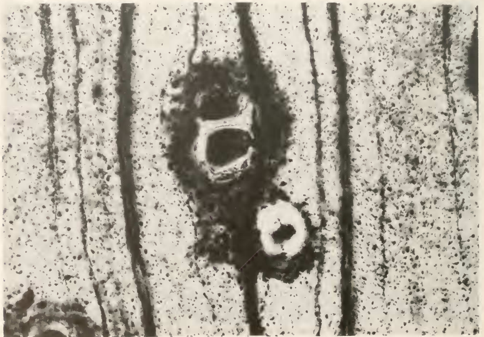
Fig. 6: Cross section. Rays, axial parenchyma confluent, thickwalled fibres. \times 133 .
